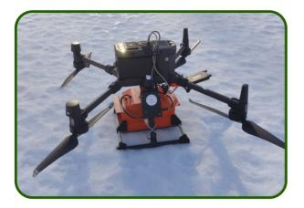
Zond Aero 1000 is an ultra light weight single-unit GPR, specially designed for portable solutions. Device could be used as the standalone on-board equipment with the powering from external source and Ethernet cable connection or inside of the fully protective case with its own built-in Lithiumlon battery and WiFi.
